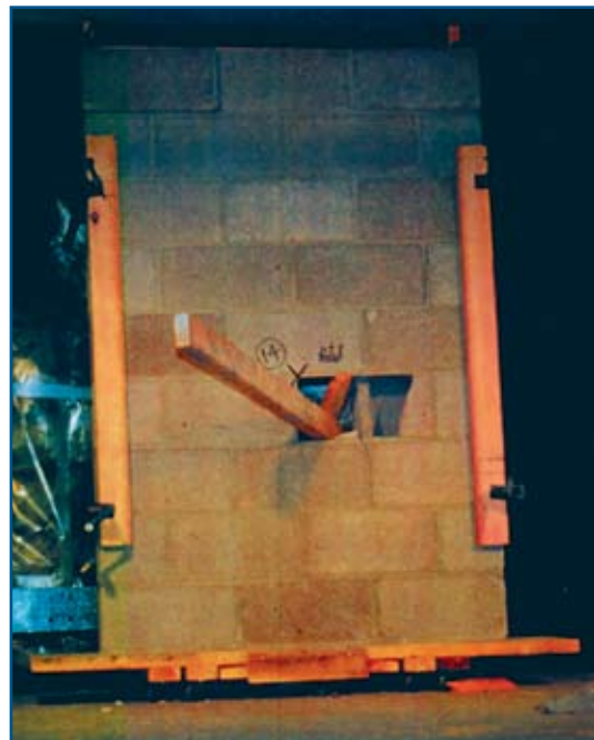
2" x 4" wood stud launched at 100 mph pierces unreinforced masonry wall, WERC, Texas Tech University
